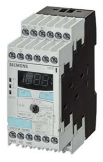
TEMPERATURE MONITORING RELAY THERMOCOUPLE J,K,T,E,N,S,R,B, 2 THRESHOLDS, DIGITAL, -99 DEGREES C TO 1800 DEGREES C (SENSOR-DEPENDENT), 24 V TO 240 V AC/DC, 2 X 1 CO + 1 NO, WIDTH 45 MM, SCREW TERMINAL
