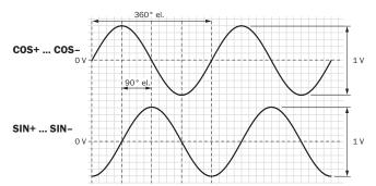
Signal diagram with read head moving in direction of arrow at 120  $\Omega$  load with US = 5 V
