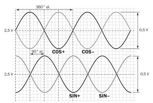
Signal diagram with read head moving in direction of arrow at 120  $\Omega$  load with US = 5 V Signal SIN/COS after differential generation
